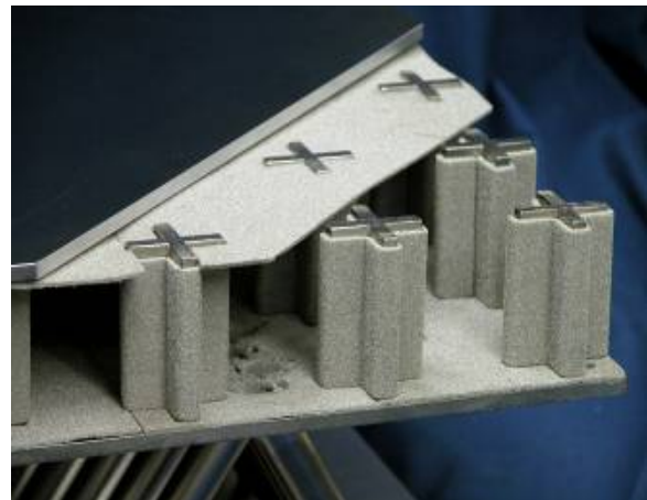
Figure 2: Digital picture of an opened heat spreader plate with nickel foam wicking visible on the cross structures [2].
