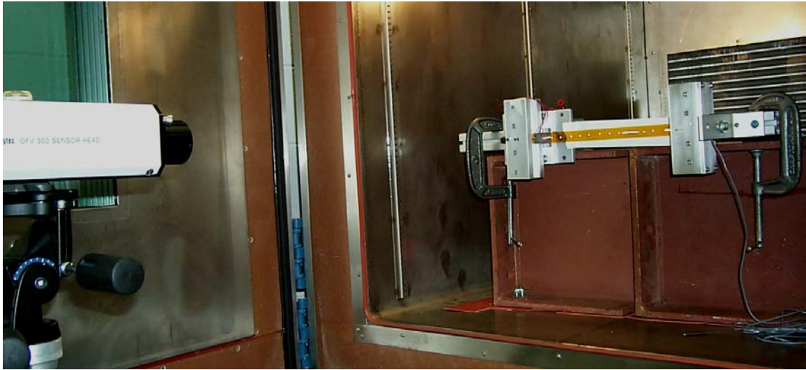
Figure 3. Photograph of the test setup, highlighting the laser vibrometer sensor and the Kapton sample test rig sitting inside of the Tenney Environmental chamber.
