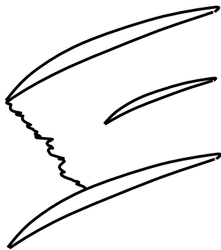
Figure 6: Shock System as Visualized by Wennerstrom
