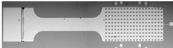
Figure 1: Evaporated thin film specimen, gauge truncated [taken by author]
