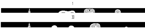
Figure 6: Fingerprints generated from the start (1) and end (30) of the corrosion study by the DWFT.
