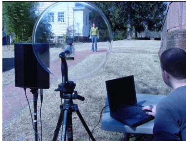
Figure 1. Picture showing the experimental nonlinear acoustic concealed weapons and explosives detection apparatus.
