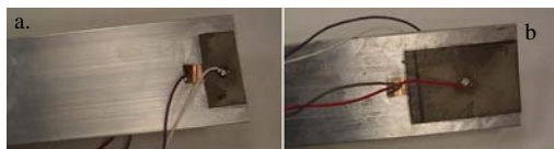
Figure 1. a) PZT 1, b) PZT 2 (attached to same end, opposite side of beam).
